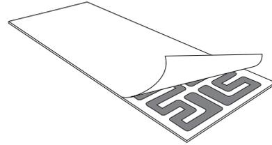
This element type, created by acid etching a circuit in nickel alloy resistance foil, is available in silicone rubber and polyimide heater types. The etched foil element is noted for its excellent circuit pattern repeatability and superior heat transfer, which results from greater area coverage of the element. Other benefits include:
