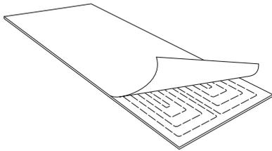
Available on silicone rubber heaters, this element style is created by spiraling fine resistance wires around a fiberglass cord. The element is then laid out in a pattern designed specifically for a specific application. The benefits of wire-wound elements include:
